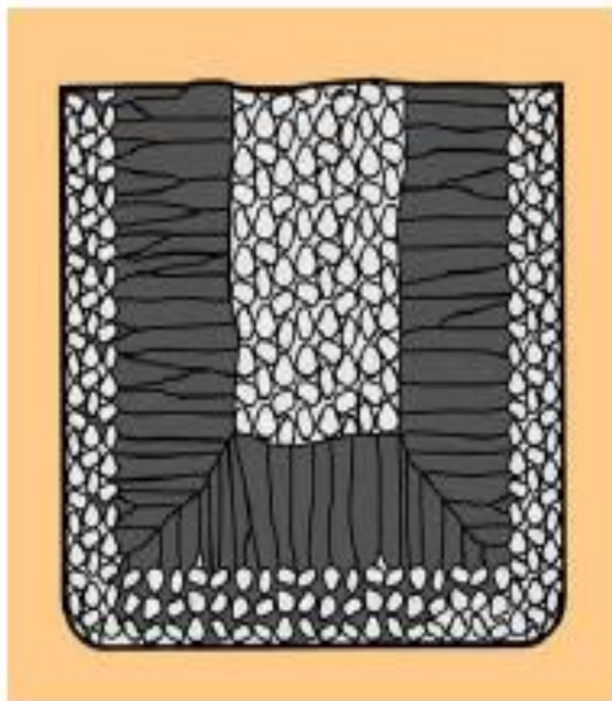
Figure 10.7 - Characteristic grain structure in an alloy casting, showing segregation of alloying components in center of casting
